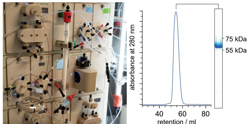
**Figure 1.** *Left:* Most recombinant protein purifications are performed using various fast protein liquid chromatography systems (FPLCs) in the facility. *Right:* Elution profile of a recombinant protein during the final gel filtration step, showing the absorbance at 280 nm over the column volume (retention). The purity of the protein is visualised by Coomassie-stained SDS-PAGE next to the elution profile.
