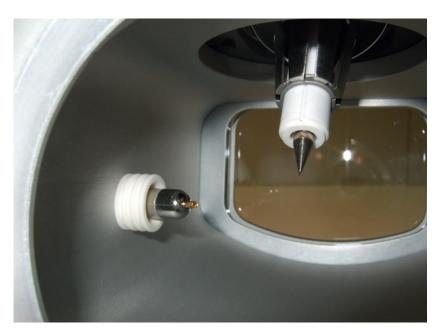
**Figure 1.** The inside of an electrospray ionization (ESI) source showing ESI needle (upper right) pointing towards the mass spectrometry entrance. A fluid sample is transferred to the gaseous phase by the application of high voltage resulting in a fine spray. The same source housing can be modified for other ionization methods. Corona discharge needle (lower left) is necessary for atmospheric pressure chemical ionization (APCI).
