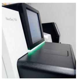
Figure 1. NextSeq 500 benchtop, high throughput sequencer from Illumina.
