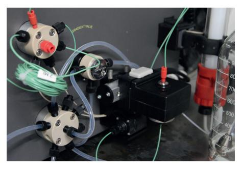
Figure 1. Side view of the Äkta Prime Plus Chromatography system, showing inlet, injection and gradient valves, as well as the UV and conductivity monitor.
